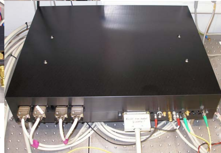
Prototype of a 216 MHz laser and a small distribution unit. The second iteration is on its way.
