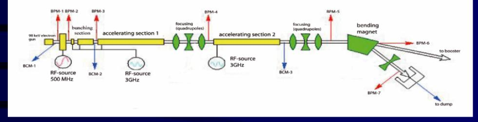
•electron accelerator used as injector for the SLS storage ring
