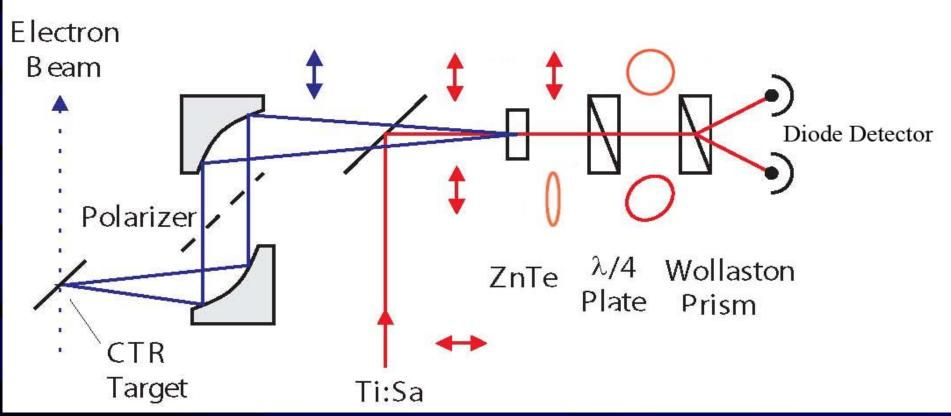
•Laser and CTR are horizontally polarized
