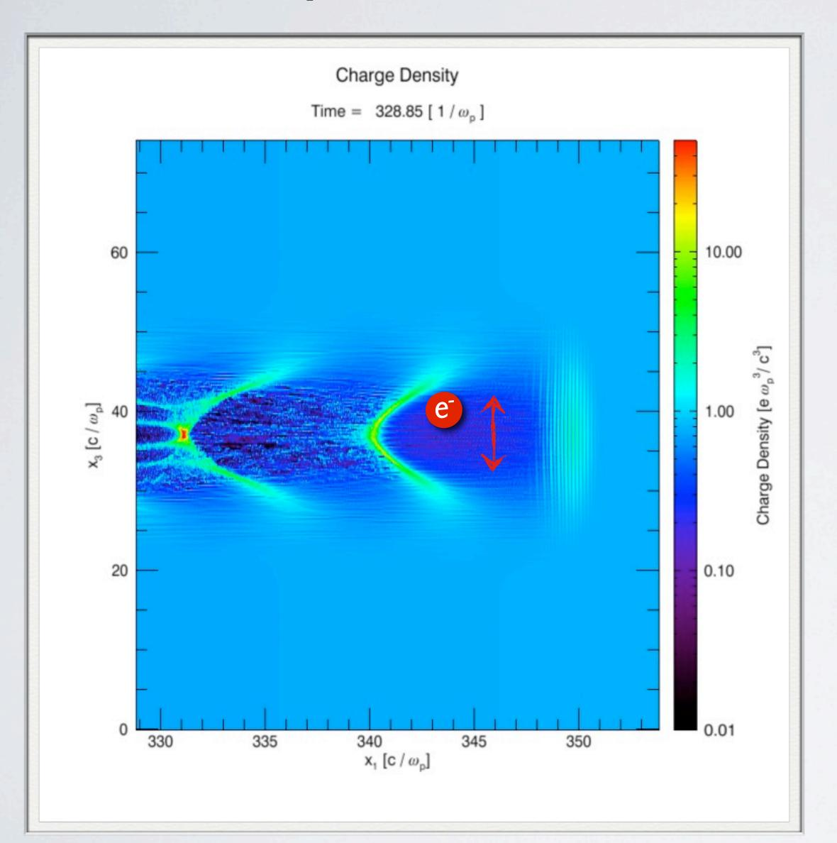
Control transverse offset between laser pulse and electron bunch for tailored betatron sources
